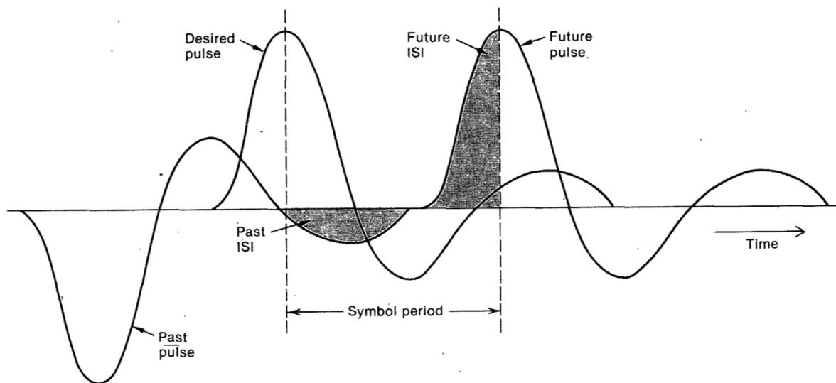
Fig. 4. Received pulse sequence after channel filtering.
