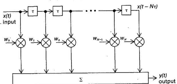
Fig. 1. Tapped-delay line (TDL) filter.
