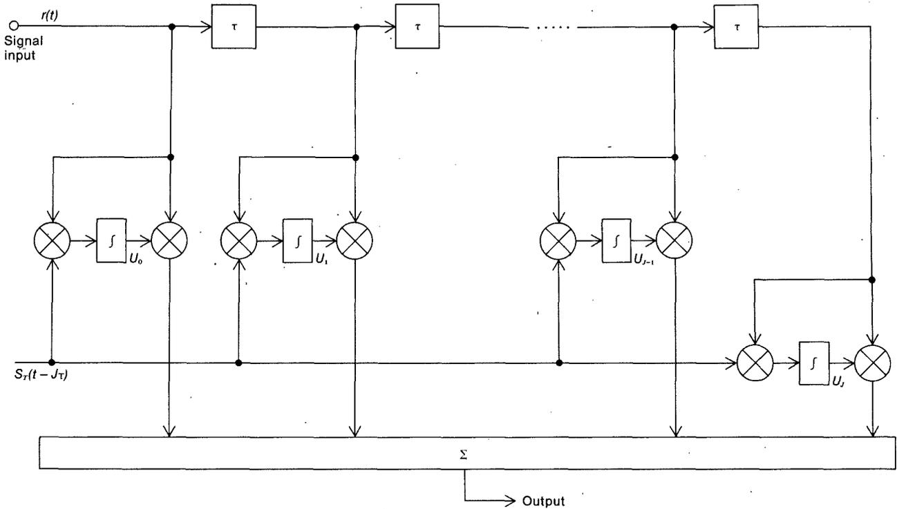
Fig. 2. RAKE filter
